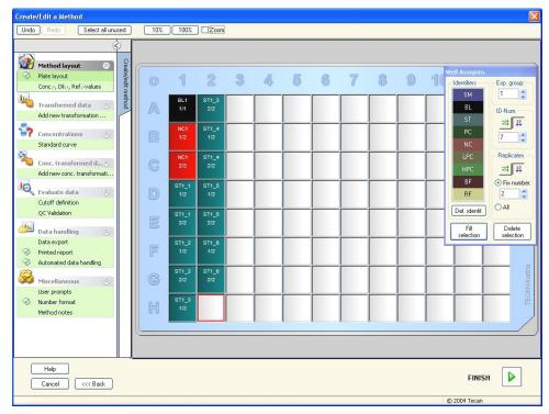
Click **Select all unused** from the toolbar to select all empty wells on the plate. Then hold down the control (Ctrl) key and click the well **H12**, so that it remains blank and unmarked.
