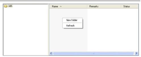
In the **Save** window, the folder, specified by the default path of the method, workspace, standard curve or sample ID list, is opened automatically, whenever a new file is created. If an already existing file is modified, the path to the current location of the file will be opened. However, it is only possible to save files in the default folder, or in an existing or newly created subfolder within this folder.
