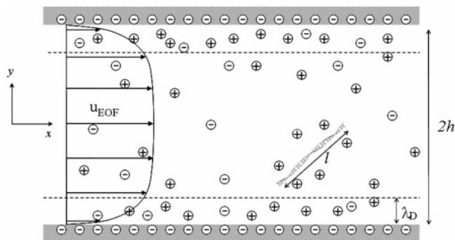
**Figure 1.** Schematic of nanochannel electrophoresis of rodlike oligonucleotides. Important length scales are the depth of the channel ( $2h$ ), the length of the dsDNA ( $l$ ), and the Debye length ( $\lambda_D$ ).
