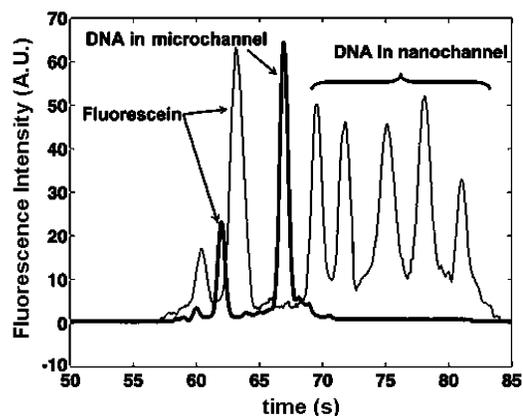
**Figure 3.** Electropherograms for free-solution DNA separation experiments in a 50  $\mu\text{m}$  deep microchannel (thick line) and a 100 nm deep channel (thin line). The BGE concentration and applied field for both were 10 mM and 100 V/cm, respectively. Both experiments used the same sample solution ( $\sim 167 \mu\text{M}$  dsDNA and fluorescein). The nanochannel clearly improves resolution.
