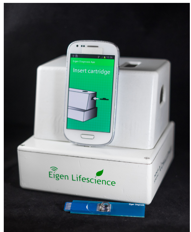
Fig. 2. The Eigen Diagnosis Platform (EDP). The EDP consists of three parts: a disposable cartridge, a reader station, and a smartphone running the Eigen Diagnosis App (shown on the smart phone screen). The reader acquires biological signals from the GMR biosensor in the cartridge, and transfers the data to the smartphone for signal processing.
