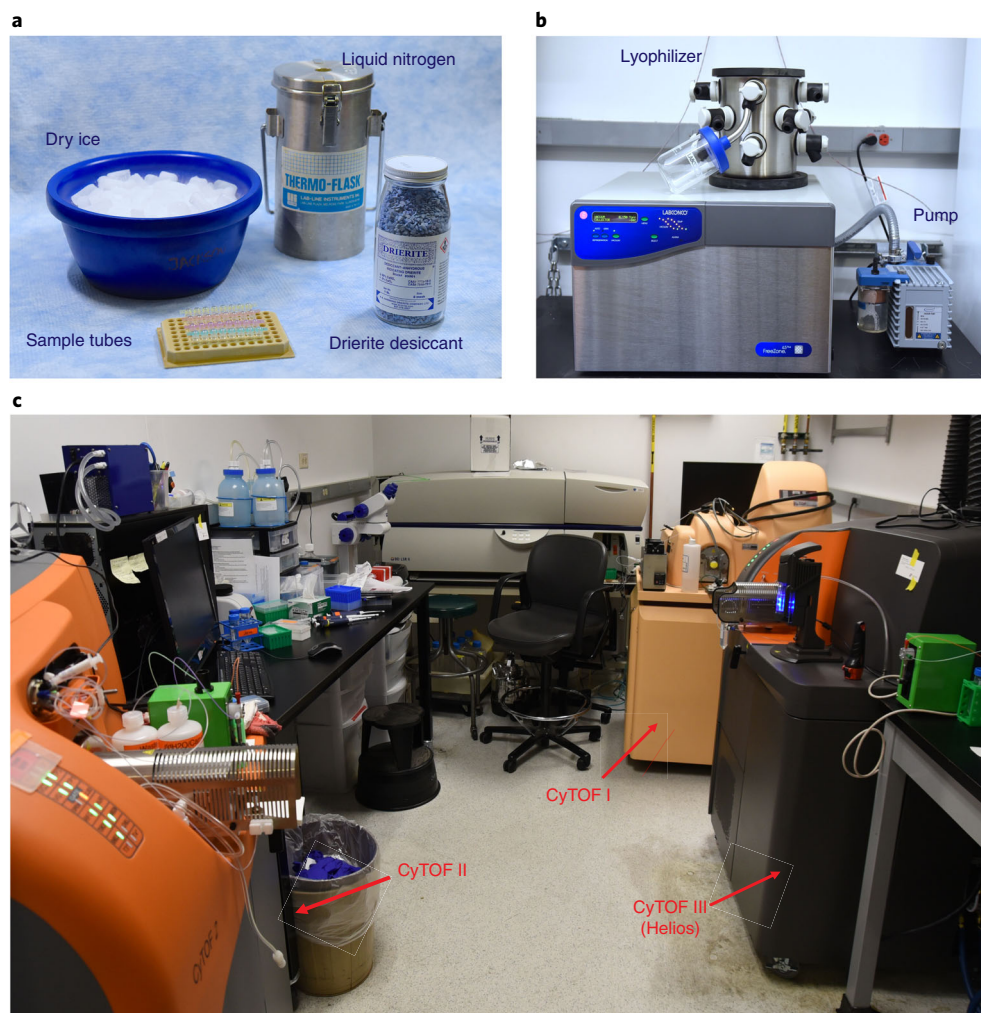
Fig. 4 | Materials and equipment. a , Liquid nitrogen tank for snap freezing of the solutions of Pd@mal-DOTA complexes, PCR tubes in a 96-well metal block, dry ice for placing frozen sample PCR tubes, and Drierite desiccant for storing dried palladium mass tags to protect them from moisture. b , Lyophilizer and pump for ice-drying of palladium mass tags. c , CyTOF instruments of v1, v2, and v3 (Helios) used in our lab.
