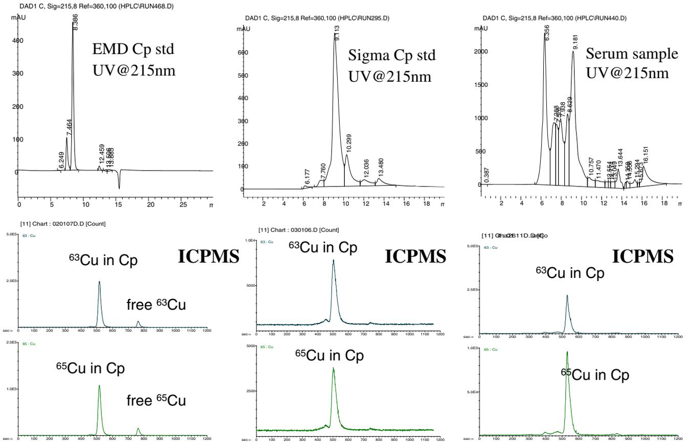
**Fig. 1** SEC-ICPMS chromatograms for Cp standards and serum sample; X axis: retention time in min for SEC and sec for ICPMS; Y axis: absorbance at 215 nm for UV chromatograms and total counts for ICPMS chromatograms
