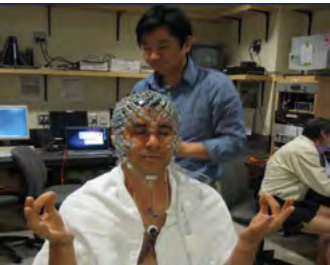
Figure 3. A scan subject is being prepared for a functional MRI scan (fMRI) that includes the MR safe EEG (electroencephalography) system (www.egi.com). Functional MRI is a type of specialized MRI scan used to measure the hemodynamic response (change in blood flow) related to neural activity in the brain or spinal cord. EEG is the recording of electrical activity along the scalp. EEG measures voltage fluctuations resulting from ionic current flows within the neurons of the brain.
