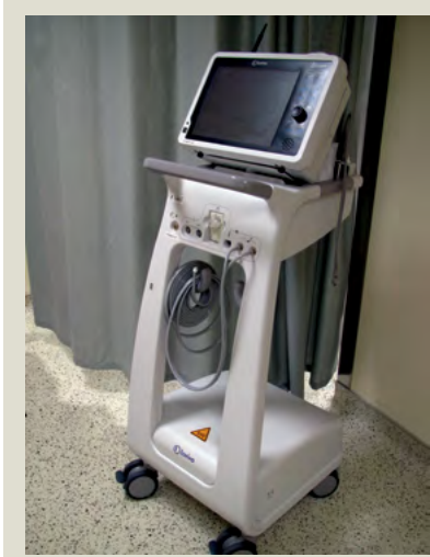
Figure 4. The new Invivo Expression physiologic monitor that includes the following options: wireless ECG (electrocardiogram), wireless SPO2 (heart rate and saturated oxygen), body temperature, invasive blood pressure, NIBP (non-invasive blood pressure), EtCO2 (end-tidal CO2), sedation and anesthesia.
