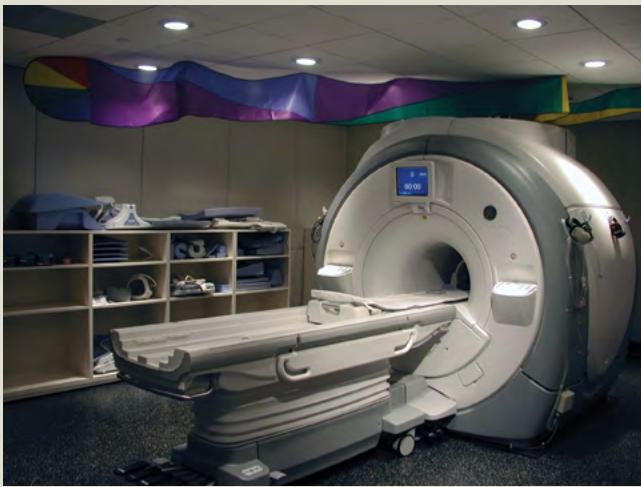
Figure 1. The ‘3T2’ at the Lucas Center is a G.E. Healthcare Discovery 750 MRI system
