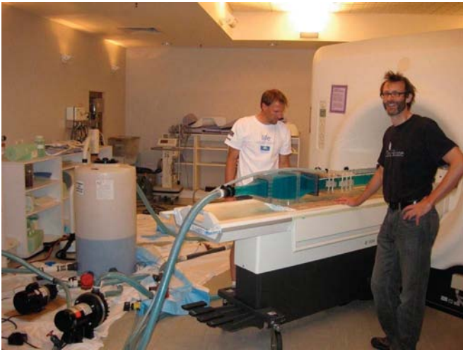
Figure 1. Marcus Alley, PhD, research associate (right), assists Chris Elkins, PhD, a researcher from Mechanical Engineering (left) with a mechanical flow phantom at the 1.5T whole body magnet. Images are generated that resolve spatially in 3 directions plus time resulting in a “4D” scan.
