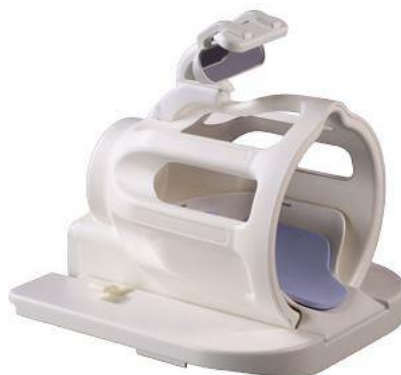
8-Channel Head Coil (where the participant will be resting his / her head)
