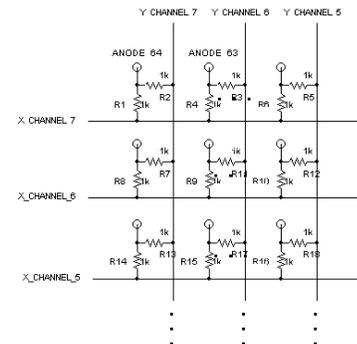
Fig. 2. Symmetric charge division replaces the conventional resistor divider scheme depicted in Fig. 1. At the end of each X or Y channel is a charge sensing preamp that collects and amplifies the charge proportional to its weight on the axis it encodes.
