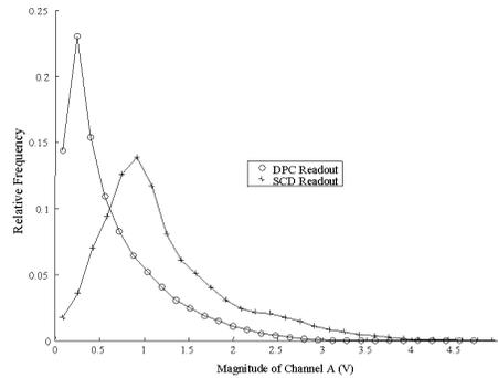
Fig. 7 The relative frequency of voltages for Channel A is shown for  $^{57}\text{Co}$  flood irradiation. Selecting the worst-case event, usually at the corner, and comparing to the average voltage determines the peak to average.
