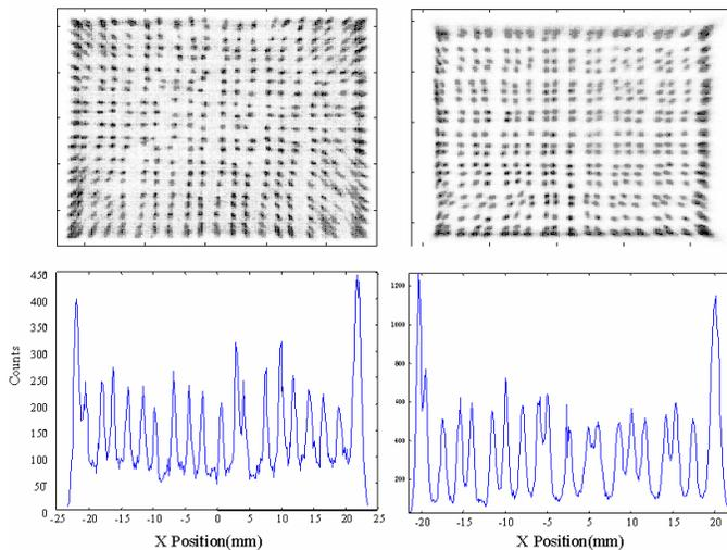
Fig. 8. Raw flood images of the LSO crystal array using the DPC(left) and SCD(right) readout with an open energy window are taken with a  $100\mu\text{C}$   $^{57}\text{Co}$  source. The bottom two plots are middle row profiles through the flood image.
