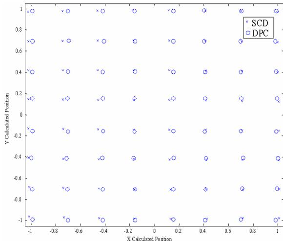
Fig.6. Each of the 64 inputs to the DPC and SCD circuits are electrically probed without the PSPMT and the position for both circuits is determined from a four-channel digitizer acquisition system and overlaid on the same plot.
