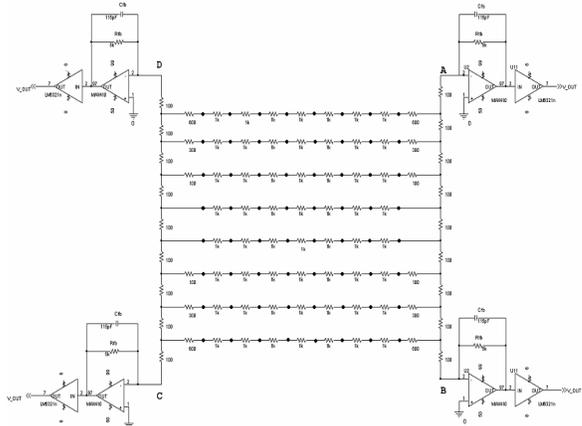
Fig. 1. A Conventional 2-D DPC network splits charge proportional to its Cartesian coordinates. This charge is collected on 4 charge sensitive preamplifiers named A, B, C, and D.
