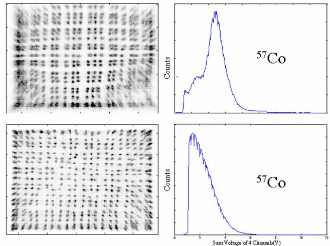
Fig. 9. Comparison of raw flood images between different gain settings for the DPC readout. Global sum energy spectra for the raw data are given on the right for each gain setting. The top image contains barrel distortion from compression artifacts created by the readout electronics, but a clear peak in the raw global energy spectrum can be seen. To avoid this saturation the amplifier gains are lowered considerably at the cost of the energy spectra as shown in the bottom row.
