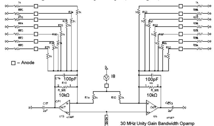
Fig. 4. A charge loss path exists from the anode to the virtual ground of the charge sensing preamp. In the example shown a charge source, I8, injects charge that is split symmetrically and collected by an X-axis and Y-axis preamp. Fourteen other anodes are connected to the same virtual ground and provide a path for charge to "leak".
