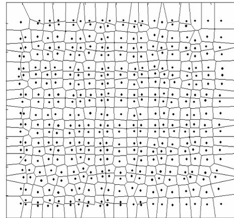
Fig. 12. Crystal map of the SCD imager is determined by selecting events that are the minimum distance to peaks identified in flood map.
