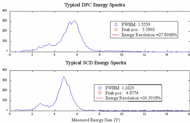
Fig. 11. Energy resolutions of a single position gated crystal from the large LSO crystal array taken from flood irradiation with a  $^{57}\text{Co}$  source. In this measurement the DPC imager electronics were optimized for energy resolution rather than spatial linearity (Fig. 10).
