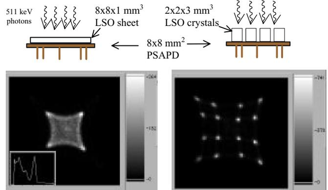
Fig. 2. 2-D histograms of positioned LSO scintillation detector events for one layer from each of the two face-on configurations depicted at the top, using an  $8 \times 8$  mm<sup>2</sup> PSAPD. Left: Flood image for 1 mm thick crystal sheet. Inset:  $^{22}\text{Na}$  energy spectrum with 12.3% FWHM energy resolution for the 511 keV photopeak. Right: Flood image for  $4 \times 4$  array of  $2 \times 2 \times 3$  mm<sup>3</sup> crystals.
