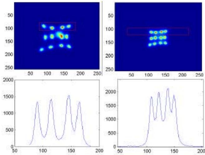
Fig. 6. Top: 2-D <sup>22</sup>Na flood histograms of the 4x3 array of 2x2x3 mm<sup>3</sup> LSO crystals side-coupled to the 8x8 (left) and 14x14 mm<sup>2</sup> (right) PSAPDs (similar to that depicted in Fig. 2, top right). Bottom: 1-D profile through top crystal rows of each flood image.
