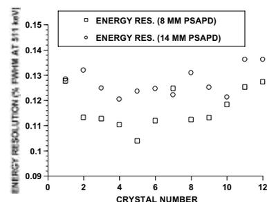
Fig. 5. Plot of 511 keV photopeak energy resolution for individual crystals of a  $4 \times 3$  array of  $2 \times 2 \times 3 \text{ mm}^3$  LSO crystals side-coupled to  $8 \times 8$  and  $14 \times 14 \text{ mm}^2$  PSAPDs (similar to that depicted in Fig. 2, top right).
