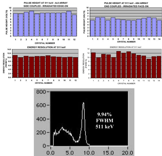
Fig. 4. Comparison between 511 keV photopeak pulse height (top plots) and energy resolution (middle plots) for individual  $2 \times 2 \times 3 \text{ mm}^3$  LSO array crystals coupled sideways (left) and end-on (right) to an  $8 \times 8 \text{ mm}^2$  PSAPD. Bottom: Best single crystal energy spectrum for the side-coupled array.
