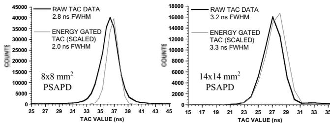
Fig. 7. Coincidence TAC spectra measured with (left) the 8x8 and (right) 14x14 mm<sup>2</sup> PSAPDs.
