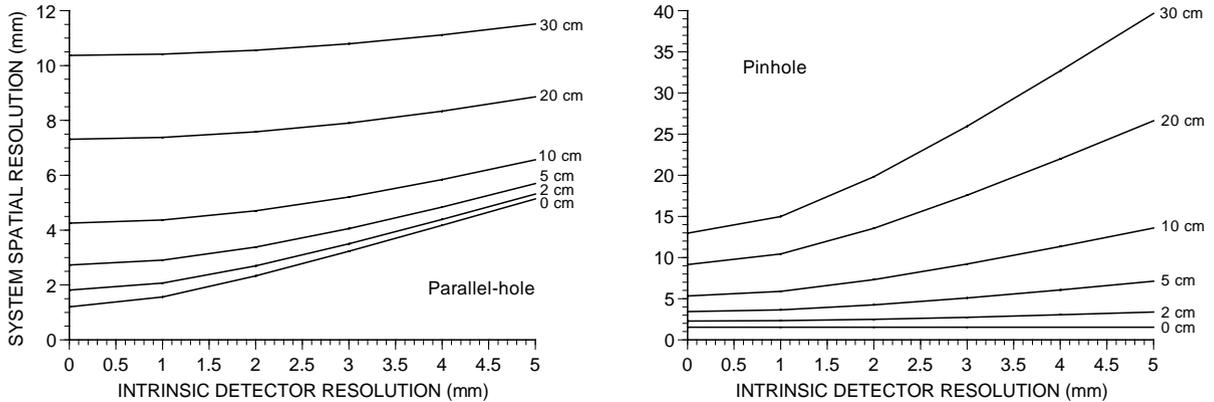
Fig. 9. Calculated spatial resolution (FWHM) as a function of intrinsic detector spatial resolution for various source-collimator distances for parallel-hole (left) and pinhole (right) collimators. We have assumed a collimator hole diameter of 1.2 mm, height of 4.0 cm, and  $\mu = 27 \text{ cm}^{-1}$  for lead at 140 keV. For the pinhole an apex angle of  $45^\circ$  and the magnification factor have been included.
