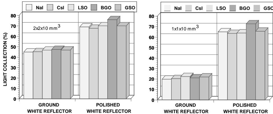
Fig. 8. Average fraction (%) of the available scintillation light collected from the ends of different length and type of scintillation crystals (1 and 2 mm wide) for two different crystal surface conditions. Even with the most ideal surface conditions, only a fraction of the light is collected. In reality, the fraction lies somewhere between that for the two surface extremes (for example, 20–60% for  $1 \times 1 \times 10 \text{ mm}^3$  LSO).
