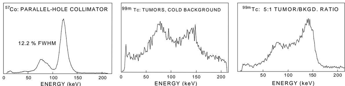
Fig. 2. Left: Point source energy spectrum. Middle: Breast phantom energy spectrum with hot tumors, cold background. Right: Breast phantom energy spectrum with hot tumors, warm background (5:1 tumor:background concentration ratio). Volume of background used:  $136\text{ cm}^3$ .
