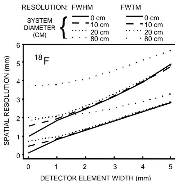
Fig. 12. Calculated  $^{18}\text{F}$  PET system spatial resolution limit (FWHM and FWTM) as a function of detector element width for various system diameters (detector separations). For 1 mm detectors and 10 cm detector separation the spatial resolution potential is  $\sim 750 \mu\text{m}$  FWHM. Adapted from Ref. [21].
