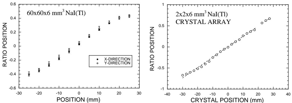
Fig. 5. Plots of the line source position measured from the resulting images as a function of its true position allows an assessment of spatial linearity for imaging with the  $60 \times 60 \times 6$  mm<sup>3</sup> continuous crystal (left) and the segmented crystal array comprising  $2 \times 2 \times 6$  mm<sup>3</sup> crystals (right). Spatial linearity is improved at the edges for the discrete array.
