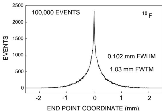
Fig. 11. Histogram of x-coordinates of 100,000 calculated positron trajectories represents the 1-D resolution blurring function for positron range. Adapted from Ref. [21].
