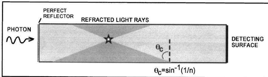
Fig. 7. Depiction of major light loss mechanism in long and skinny crystals. The poor aspect ratio means a significant fraction of the available light is lost through the crystal sides. Most of the light impinging on the crystal sides at angles less than the critical angle (shaded) will exit the crystal and not be piped down to the small detecting surface.
