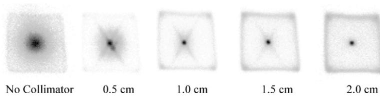
Fig. 3. Images of a  $^{57}\text{Co}$  point source using a 6 cm FOV NaI(Tl)-PSPMT camera for different LEHR collimator thickness varying from 0 to 2.0 cm. The relative collimator sensitivities are from left to right: 1.00:0.113:0.016:0.011:0.009. The corresponding system spatial resolutions are 13.6, 5.7, 3.6, 3.3, and 3.3 mm FWHM, respectively. Relative scaling is used for display.
