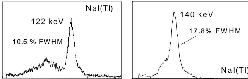
Fig. 6. Collimated point source energy resolution measured in a (left)  $60 \times 60 \times 6 \text{ mm}^3$  continuous crystal, and (right)  $2 \times 2 \times 6 \text{ mm}^3$  discrete crystal from a crystal array.
