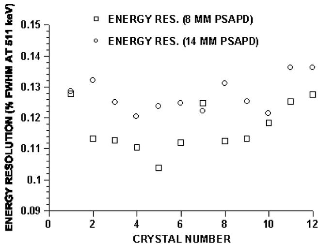
Fig. 5. Plot of 511 keV photopeak energy resolution for individual crystals of a  $4 \times 3$  array of  $2 \times 2 \times 3$  mm<sup>3</sup> LSO crystals side-coupled to  $8 \times 8$  and  $14 \times 14$  mm<sup>2</sup> PSAPDs (similar to that depicted in Fig. 3, top right).
