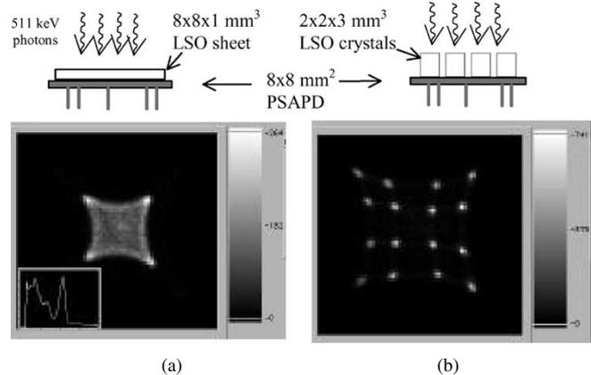
Fig. 2. Two-dimensional histograms of positioned LSO scintillation detector events for one layer from each of the two face-on configurations depicted at the top, using an  $8 \times 8$  mm<sup>2</sup> PSAPD. (a) Flood image for 1 mm thick crystal sheet. Inset: <sup>22</sup>Na energy spectrum with 12.3% FWHM energy resolution for the 511 keV photopeak. (b) Flood image for  $4 \times 4$  array of  $2 \times 2 \times 3$  mm<sup>3</sup> crystals.
