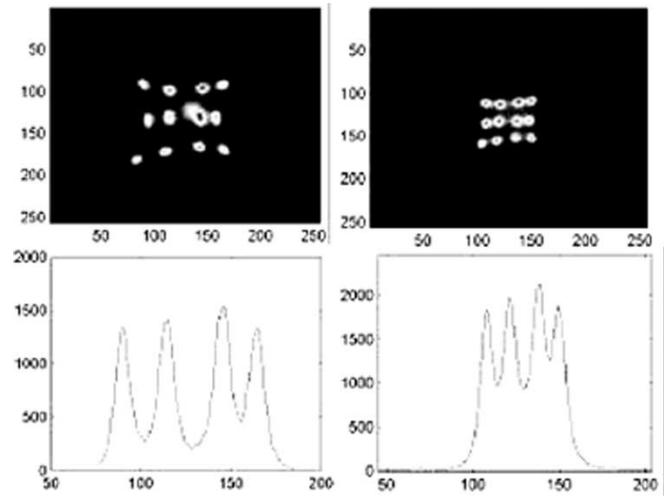
Fig. 6. Top: 2-D <sup>22</sup>Na flood histograms of the  $4 \times 3$  array of  $2 \times 2 \times 3$  mm<sup>3</sup> LSO crystals side-coupled to the  $8 \times 8$  (left) and  $14 \times 14$  mm<sup>2</sup> (right) PSAPDs (similar to that depicted in Fig. 3, top right). Bottom: 1-D profile through top crystal rows of each flood image.
