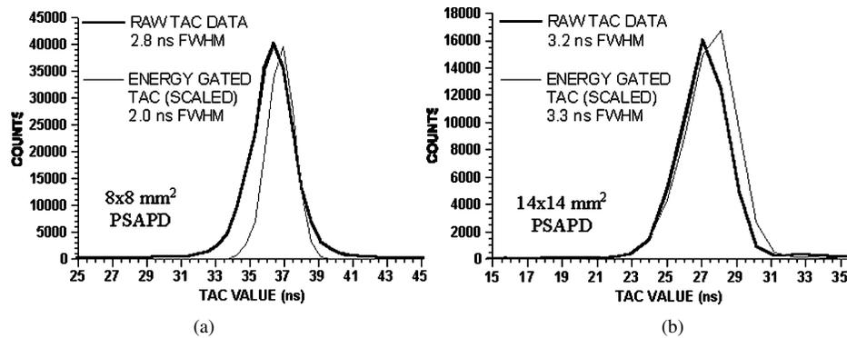
Fig. 7. Coincidence TAC spectra measured with (a) the  $8 \times 8$  and (b)  $14 \times 14$  mm<sup>2</sup> PSAPDs. The fitting errors in the quoted resolutions are  $\pm 0.1$  ns.
