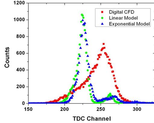
Fig. 5: The timing spectra for all three methods. A narrower peak means the better time resolution. The peak offset between the digital CFD and the other two other models is caused by the delay applied in the CFD algorithm.
