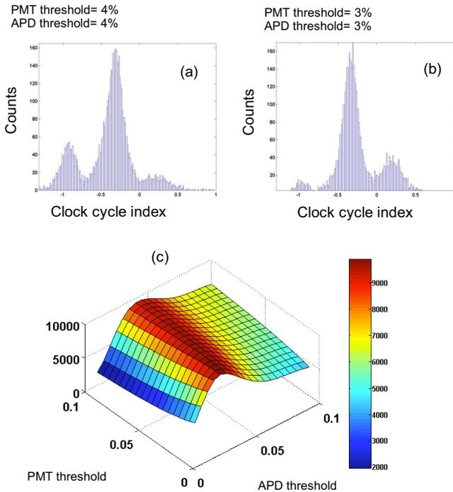
Fig. 4: (a) and (b): The coincidence timing spectrum for different threshold selection. X-axis is in clock cycle index. Y-axis is in counts. The total counts is 10000. (c) Illustration of the optimization routine for threshold determination. The threshold refers to the percent of the peak amplitude of a given raw input signal.
