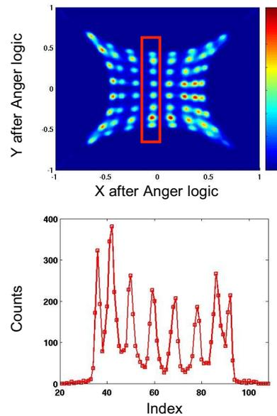
Fig. 6: (Top) Crystal identification ( $1 \times 1 \times 1 \text{ mm}^3$  LSO crystals in an 8 by 8 array. No reflector between crystals was used. Counts: 150, 000. Image size:  $128 \times 128$ . (Bottom) The central column in the image (inside the red rectangular) was used to calculate the crystal peak to-valley ratio.
