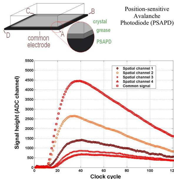
Fig. 1: For a PSAPD, the top common channel is used for extracting energy and time information. Four spatial channels (A-D) are used for position information. Raw waveform capture of five PSAPD channels is shown. The sampling rate is 108 MHz. Such digitized waveforms were used for further processing.
