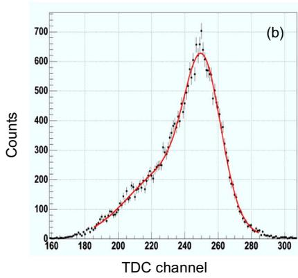
Fig. 3: (a) An example of components needed for digital CFD algorithm. (b) The coincidence time spectrum for digital CFD algorithm.  $D = 1$ .  $f = 0.03$ .  $L = 2$ . Due to different timing responses of PMT and PSAPD, the spectrum was not symmetric and was fitted by the sum of two Gaussian functions. Time-to-digital converter (TDC) channel corresponds to the bin index of the histogram of timing spectrum in the post-processing.
