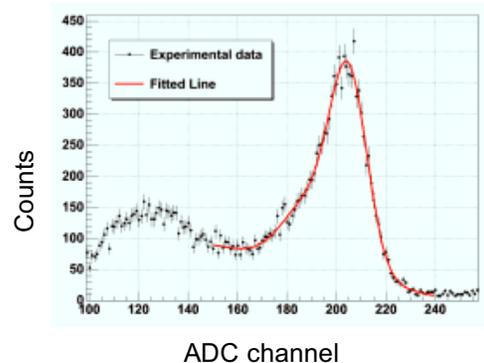
Fig. 2: The global energy spectrum of the LSO array coupled to the PSAPD extracted from the common contact. The X-axis is in ADC channels and Y-axis is in counts.
