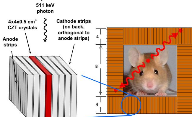
Fig. 3. Shown is a schematic of the small animal CZT system. The  $4 \times 4 \times 1/2$   $\text{cm}^3$  CZT detector has cross-strip anodes and cathodes and can position Compton scatter interactions in three dimensions. The detector is oriented in an edge-on configuration for higher sensitivity so that incoming photons see a minimum of 4 cm of CZT.
