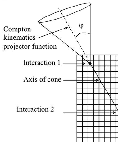
Fig 1. A schematic of Compton kinematics is shown for the 3-D CZT detector. The spatial location of two interactions in the detector determines the axis of the cone. The measured energy of the interactions determines the angle of the cone.
