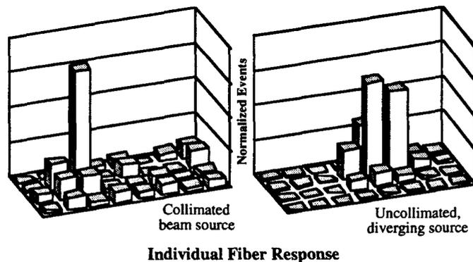
Figure 6. Probe response to collimated and diverging 1 mm beta sources.  $925 \mu\text{m}$  diameter fibers, center spaced 1.27 mm, are represented by square pixels here. Dead space is depicted.
