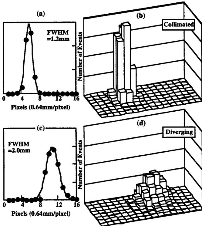
Figure 7. Interleaving technique fills dead space. The same sources as Fig. 6 are more finely sampled. In (b) & (d) the number of events are normalized and 4 boxes are equivalent to one fiber of the probe. In (a) & (c) cuts from (b) & (d), respectively, are fit to Gaussians. Full width half maximum are given.
