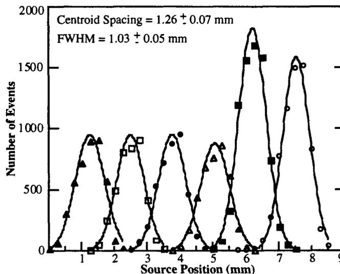
Figure 5. Point spread function of probe. Mean FWHM and centroid spacing are indicated. Error bars on these data are the size of the data points.
