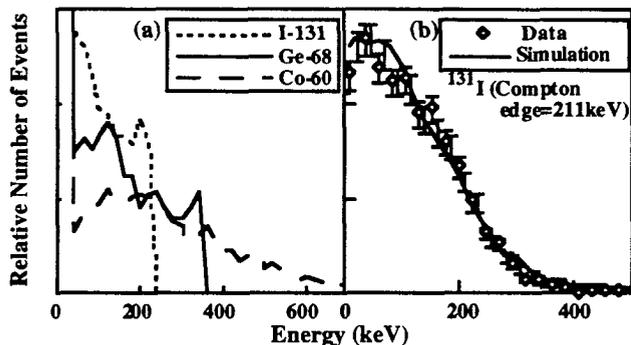
Figure 4. (a) Simulated energy deposition from the indicated sources in the scintillating fibers of the probe, i.e. the best spectra the probe could produce. No light transport is included here. Compton edges are visible for the lower energy sources, but not for  $^{60}\text{Co}$  which emits gammas at 1170 & 1330 keV. (b) Simulation of a realistic detector system with finite resolution compared to acquired data spectrum.
