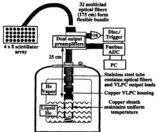
Figure 1. Components of the beta imaging intra-operative probe. A small liquid helium dewar is used to cool VLPCs which operate at about 7 degrees K in the vapor above the liquid.
