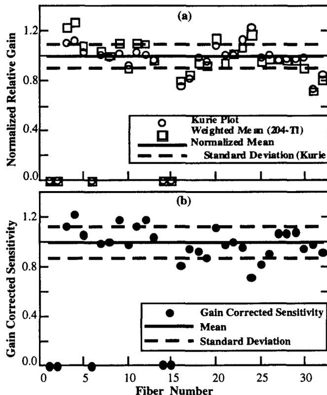
Figure 3. (a) Gain variation of the 32 element probe. Normalized results from both Kurie plot and weighted mean analyses for  $^{204}\text{Tl}$  are seen. (b) Gain corrected sensitivities of the individual fiber elements. Five dead channels are seen on the x-axes.
