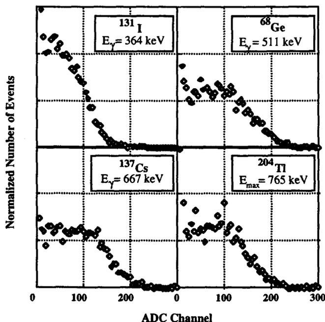
Figure 2. Spectra of 3 gamma sources and a beta source ( $^{204}\text{Tl}$ ) acquired with channel 11 of the prototype beta-imaging intra-operative probe.
