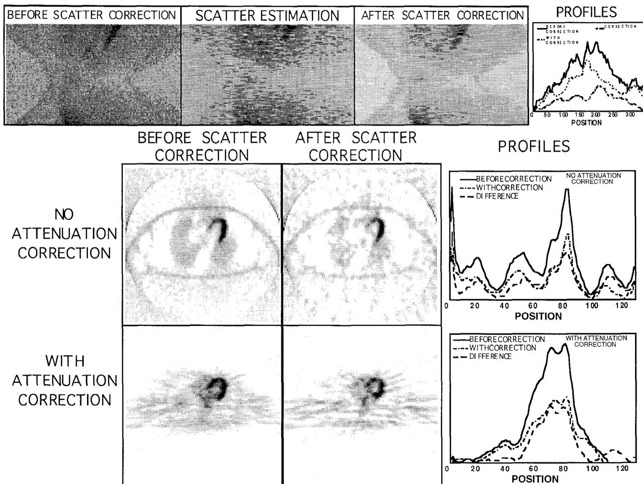
Fig. 4. Top: Uncorrected emission sinogram, Monte Carlo calculated scatter distribution and scatter corrected emission sinogram; Bottom: Corresponding reconstructed image plane with and without attenuation. Profiles through row 50 (angle 50 in sinogram and row 50 of images) are shown. There were no significant negative values.
