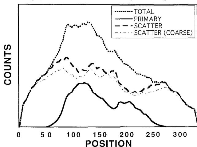
Fig. 4. Profiles through the sinograms of the Monte Carlo calculated uncorrected, corrected and scatter distributions (fine and coarse input) for a 3-D human thorax study (Legend shown at top); there were no significant negative values. The calculated scatter distributions for the coarse and finely sampled cases compare well.
