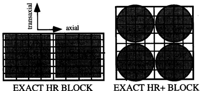
Fig. 1 Scale drawing of HR and HR PLUS detector blocks showing PM tubes superimposed on crystal matrix.
