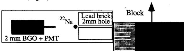
Fig. 5 Set-up used for measuring the PSF in the block.
