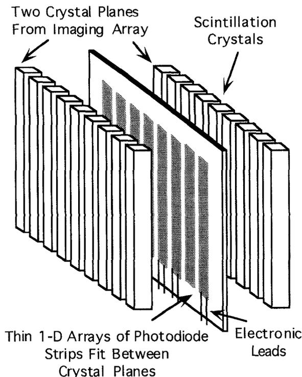
**Figure 1.** Schematic of a potential photodiode readout of a scintillation crystal array (only two crystal planes shown). The thickness of 1-D array of photodiode strips can be made  $< 250\mu\text{m}$  to minimize the dead area between crystal planes.
