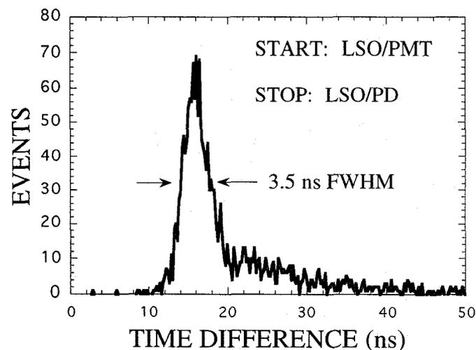
**Figure 4.** Measured coincident timing spectrum. Start:  $4 \times 4 \times 10 \text{ mm}^3$  LSO crystal on a PMT. Stop:  $2.5 \times 2.5 \times 20 \text{ mm}^3$  LSO crystal on a photodiode. A coincidence timing resolution of 3.5 ns FWHM was measured indicating good timing capability for PET with a photodiode readout.
