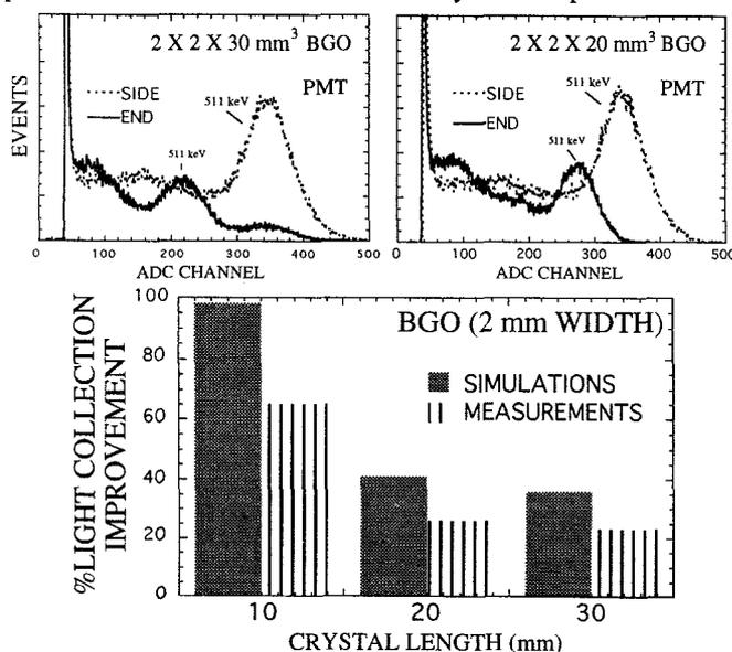
**Figure 3.** Top:  $^{22}\text{Na}$  spectra measured with  $2 \times 2 \times 20 \text{ mm}^3$ , and  $2 \times 2 \times 30 \text{ mm}^3$  BGO and PMT for side and end readout. See Figure legends. Below: Comparison between simulations and measurements of light collection improvement of side over end readout.
