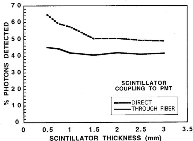
Fig. 5. Simulated light yield vs. scintillator thickness (2 mm diameter plastic).  $\text{CaF}_2(\text{Eu})$  showed the same trend. The clear fiber coupling (5 cm) removes the dependence of light yield on thickness. The 1.25 cm diameter scintillators with or without coupling to a fiber bundle, showed similar trends.
