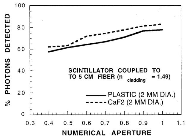
Fig. 7. Simulated scintillation light yield when coupled to a 5 cm long clear fiber as a function of the numerical aperture of the fiber.
