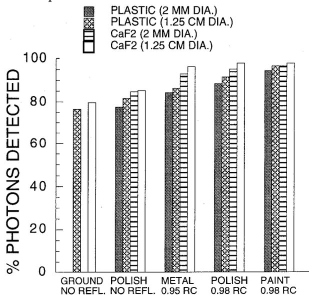
Fig. 4. Simulated scintillation light yield for various top surface treatments (RC=reflection coefficient) for plastic and  $\text{CaF}_2(\text{Eu})$  scintillators of 1.2 and 0.7 mm thick, respectively. Diameters are shown at top. For the metal reflector case, a polished surface is assumed. The best top surface treatment found was ground and painted with a diffuse reflector with a high RC (far right).
