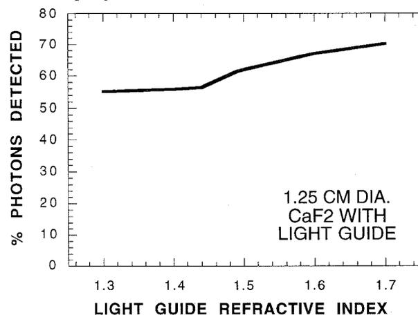
Fig. 8. Simulated scintillation light yield of a 1.25 cm diameter, 0.7 mm thick  $\text{CaF}_2(\text{Eu})$  disk coupled to a 2 mm thick light diffuser as a function of light diffuser index of refraction (no fibers).
