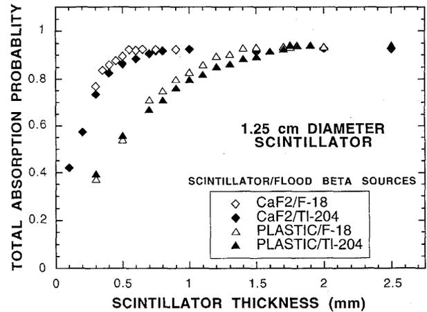
Fig. 2. Total absorption probability for beta events (trajectories) from  $^{18}\text{F}$  and  $^{204}\text{Tl}$  sources in  $\text{CaF}_2(\text{Eu})$  and plastic scintillators (a 1.25 cm diameter detector is assumed).
