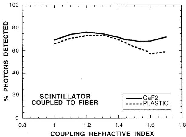
Fig. 6. Simulated scintillation light yield as a function of refractive index of the optical coupling compound used to couple a 2 mm diameter scintillator (with or without cladding) to fibers.
