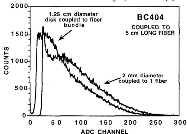
Fig. 14. Measured comparison between segmented scintillator and continuous positioning designs (BC404, 1.25 mm thickness, 2 and 12.5 mm diameters). Because the fiber bundle coupling has some light transmission dead area in the continuous design, the light output for the segmented array is higher (see Fig. 1).
