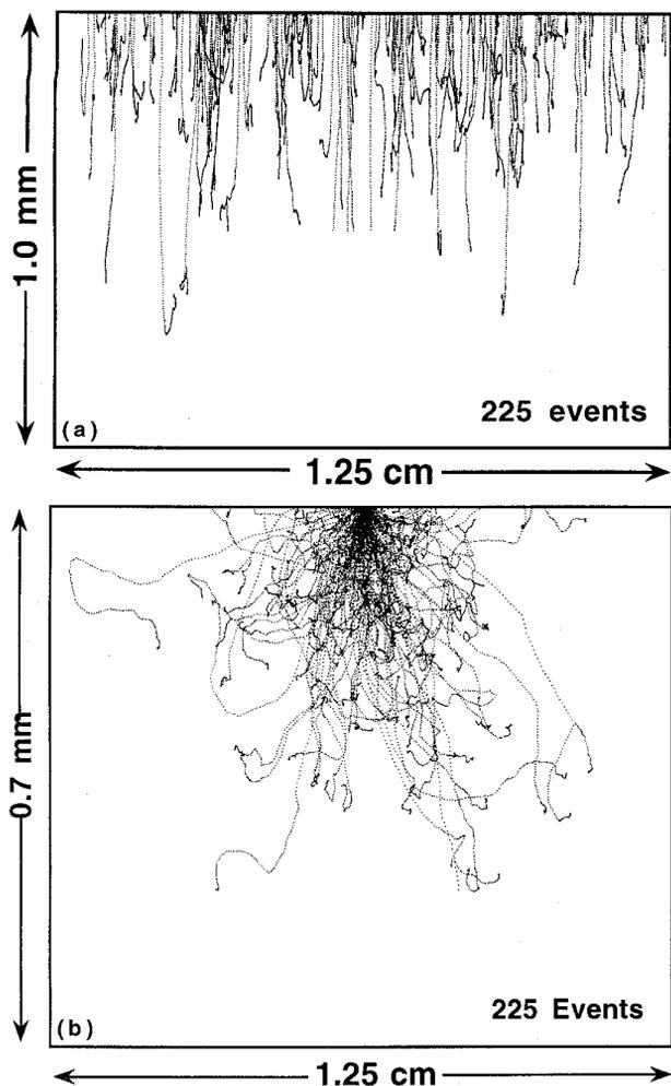
Fig. 3. Two dimensional plot (not to scale) of a Monte Carlo simulation of electron trajectories in  $\text{CaF}_2(\text{Eu})$  for (a)  $^{204}\text{Tl}$  ( $E_{\text{max}} = 765$  keV) flood source and (b)  $^{18}\text{F}$  ( $E_{\text{max}} = 635$  keV) point source at top center of scintillator. Note the effect of multiple scattering in the beta trajectories. The figures are not to scale.
