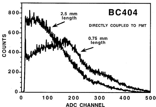
Fig. 10. Typical beta spectra measured in 0.75 and 2.5 mm lengths of 2 mm diameter BC404 scintillator directly coupled to a PMT. The relative light yield is measured by the spectrum weighted mean.
