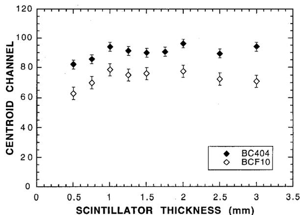
Figure 12. Light output measured for 2 mm diameter plastic scintillators coupled via a 5 cm length of clear fiber to a PMT as a function of scintillator thickness.
