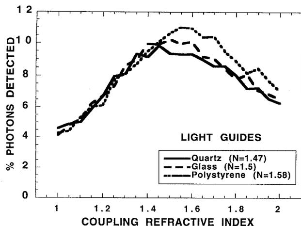
Fig. 9. Continuous detector scintillation light yield as a function of refractive index of light diffuser/fiber interface for different light diffuser materials.
