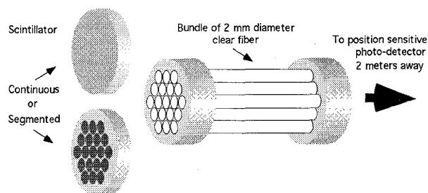
Fig. 1. Schematic of front end of the proposed Beta-Ray Camera. For flexibility, the scintillation light will be guided by a second-stage bundle of smaller diameter (< 1 mm) fibers (not shown). The total scintillator diameter is ~ 1.25 cm and the clear fiber bundle front end will be 5 cm long.
