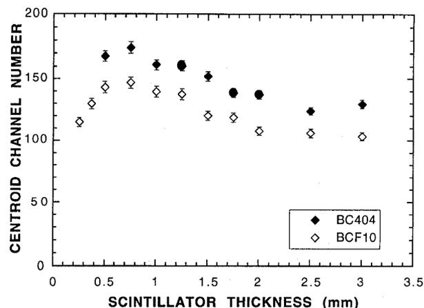
Figure 11. Light output measured for 2 mm diameter plastic scintillators directly coupled to a PMT as a function of scintillator thickness for flood beta irradiation from  $^{204}\text{Tl}$ .
