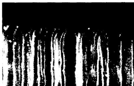
FIGURE 1. Scanning electron micrograph of the tops of a micro-columnar CsI(Tl) array similar to those used in the imaging system. Note the regularity of the  $\sim 6 \mu\text{m}$  diameter of each crystal as well as the retro-reflector like tips.
