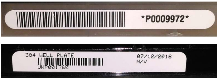
Figure: Acceptable (Top) and Unacceptable (Bottom) Barcode Sizes
