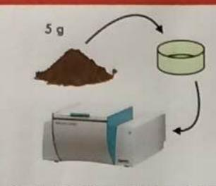
The X-Ray Fluorescence machine measures the total concentrations of a variety of metals in a single dry soil sample.
