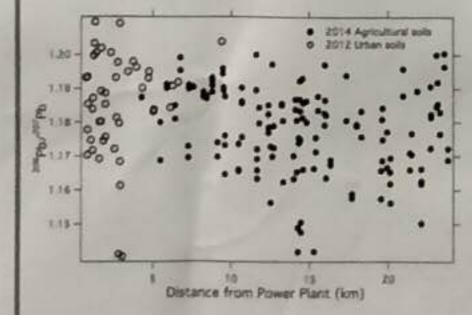
The data to the left show the ratio of Pb to Pb as a function of the sample site's distance from the Yangluo power plant. Both urban sites sampled in 2012 (within 10 km of the urban center) and agricultural sites sampled in 2014 (5 km to 20 km from the urban center) are shown. The presence of radiogenic Pb, indicated by the concentration of Pb, tends to decrease slightly with distance away from the urban center.
