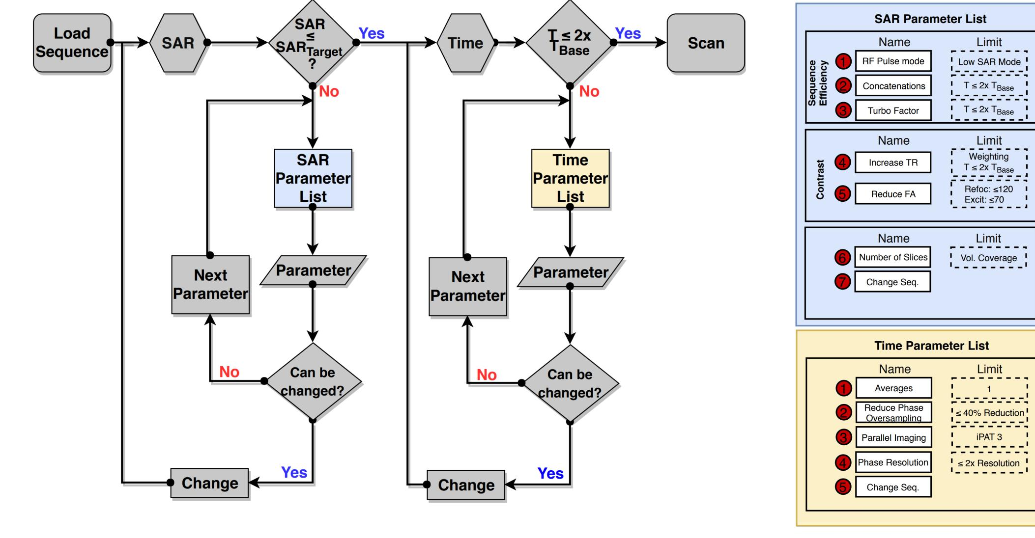
Figure 2. Workflow used for reaching a SAR target while mitigating a negative effect on image quality. Sequence parameters are modified following a given order in an sequential manner.
