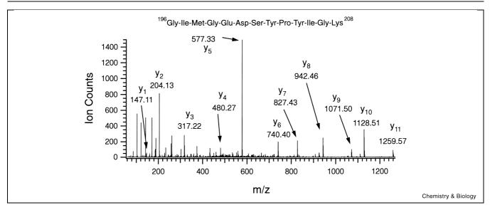
Figure 9. Low energy CID spectrum of tryptic peptides with MH+ = 1429.7. The doubly charged ion at m/z 715.35 was selected as a precursor ion. Only the C-terminal fragment ions used for sequence determination are labeled.
