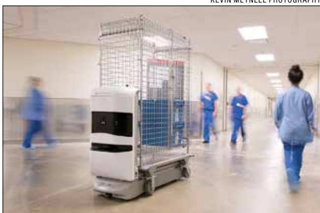
Tug robots will serve as autonomous couriers, hauling heavy loads of supplies between the central loading dock at 300 Pasteur Drive and the new hospital at 500 Pasteur Drive — a half-mile round-trip.
