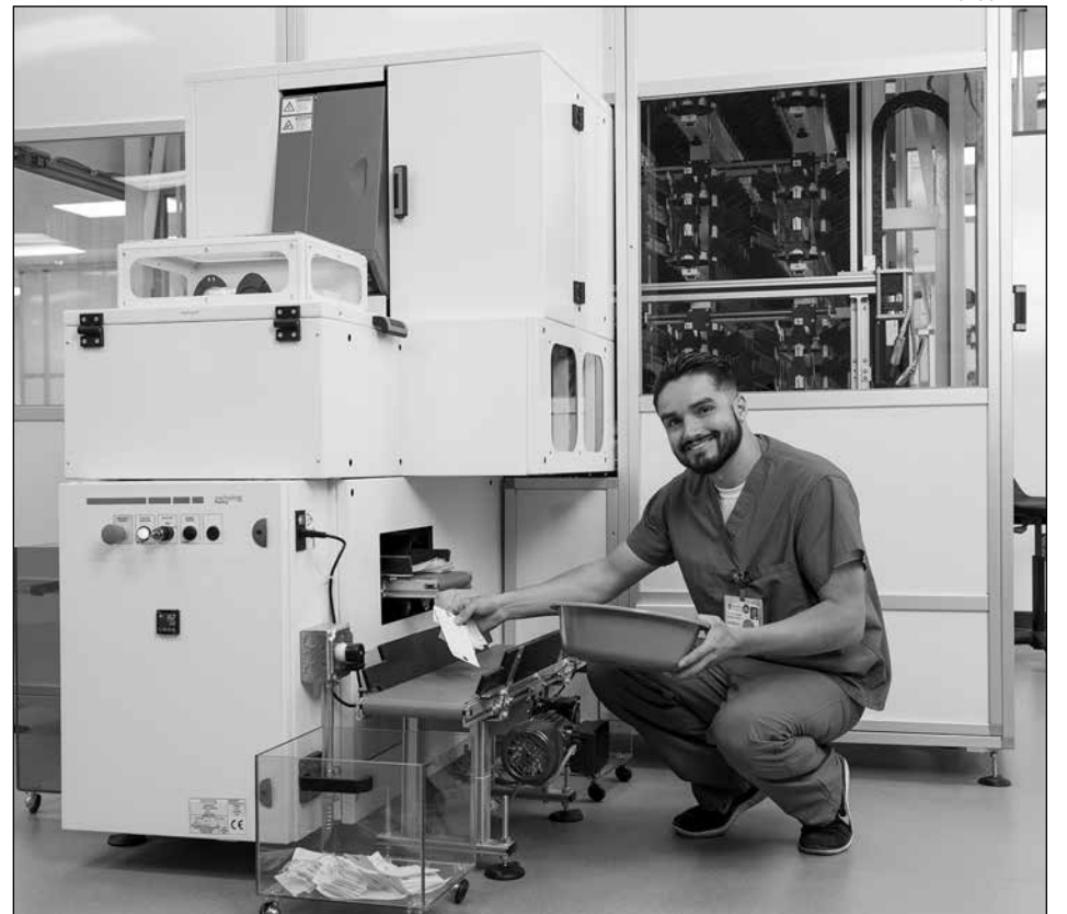
Joel Rivera, a pharmacy technician, next to the PillPick robot, which can package 1,000 doses of medicine per hour. The same work would take a technician 10 hours to complete.
