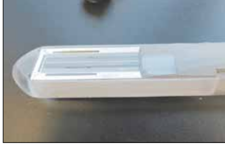
A new device employs ultrasound and photoacoustic imaging techniques to detect prostate cancer.
