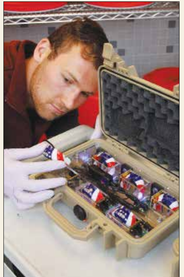
(Top) Research assistant William Mehring (right) hands a mouthguard to Menlo School sophomore J.P. McKenney. (Right) Mehring with the mouthguards, which local high school football players will wear during practices and games. The mouthguards contain sensors that measure motion in three directions.
