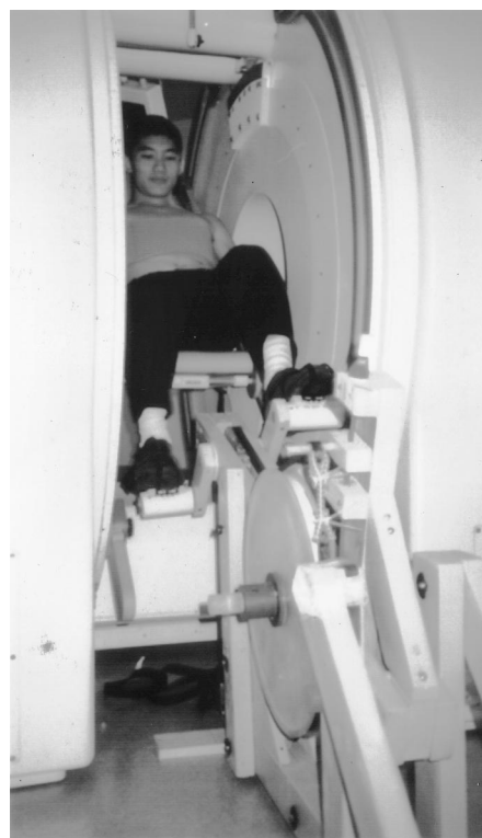
FIGURE 1. Subject pedaling on MR-compatible bicycle in 0.5 T open magnet.
