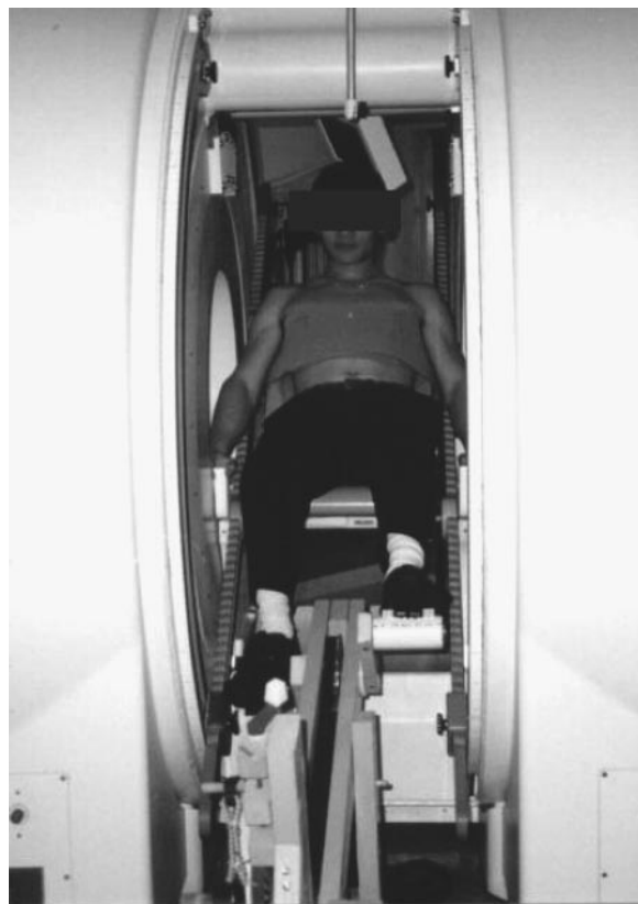
Fig. 1. A subject pedaling the custom-built magnetic resonance compatible stationary cycle with the GE 0.5-T open magnet.
