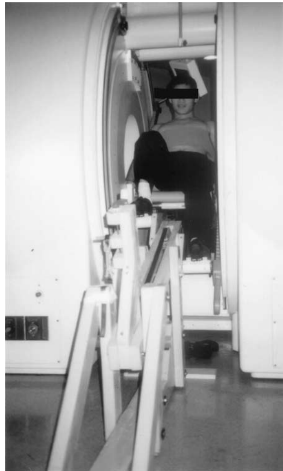
Fig 1. Subject pedaling MR-compatible bicycle in 0.5-T open magnet.
