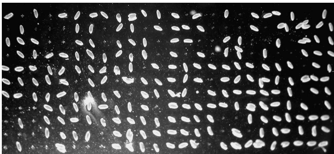
Fig. 4. An image of embryos immobilized at a sample patterned array with 200\ \mu\text{m} \times 200\ \mu\text{m} cross-shaped and 200\ \mu\text{m} \times 100\ \mu\text{m} truncated cross-shaped sites with 800\ \mu\text{m} \times 800\ \mu\text{m} pitch. The clustering is reduced substantially.
