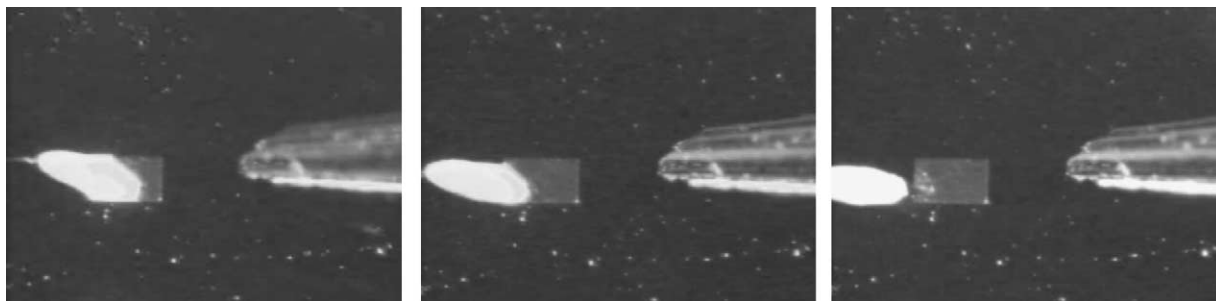
Fig. 2. A picture series illustrating the method used for measuring the adhesion force of the immobilized embryos. A water flow was imposed at an immobilized embryo by a micropipette. The flow rate at which detachment of the embryo took place was measured and a rough estimate of the drag force can be calculated using Eq. (1).
