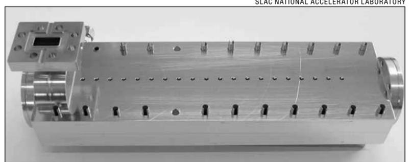
(Top) The proposed PHASER design is compact enough to fit into standard cargo containers. (Bottom) A prototype accelerator component for the PHASER project.
