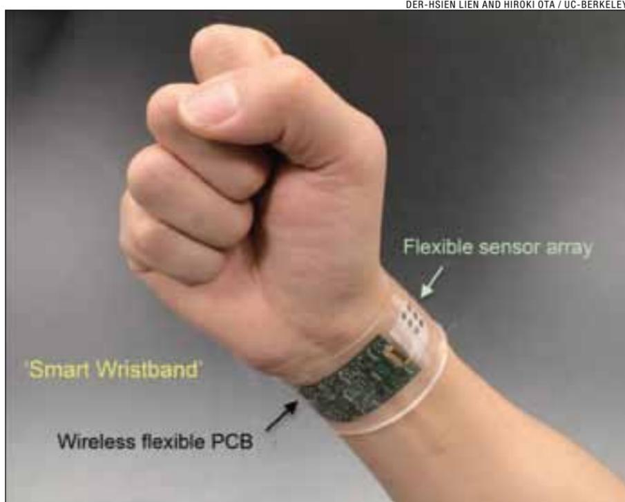
This wearable sensor measures skin temperature in addition to glucose, lactate, sodium and potassium in sweat. Integrated circuits analyze the data and transmit the information wirelessly to a smartphone or other device.
